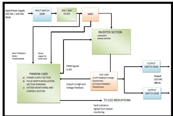
Input Switchgear section comprises of Input controlling fuses and switches used to turn ON input supply to the Frequency Converter which is then provided to input transformer of the Inverter.
