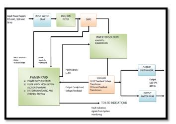
Input Switchgear section comprises of Input controlling fuses and switches used to turn ON input supply to the Frequency Converter which is then provided to input transformer of the Inverter.
