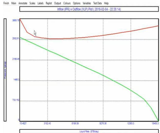
Diagram-5 : IPR VS VLP curve prior to gas injection)
