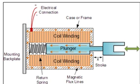
Fig. 2- Simple Solenoid
