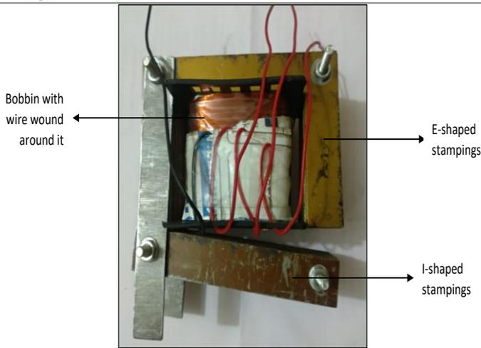
Figure 7- Solenoid Coil
