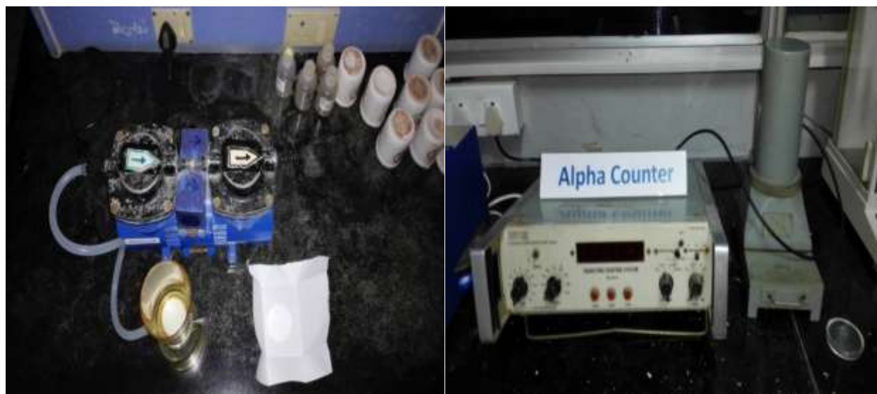
Fig 5 showing the set up of the air flow meter and alpha counter
