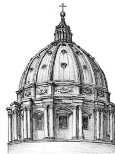
Fig.2- The dome of St. Peter's Cathedral. The shape symbolized heaven and due to structural considerations it was slightly elongated.
