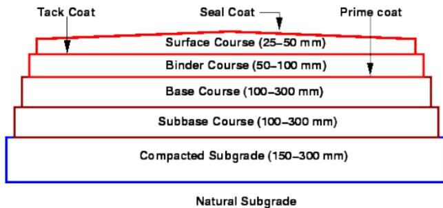
Fig.2 Cross-section of a flexible pavement
