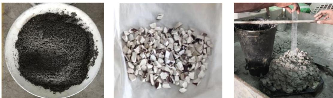
**Figure 1 Constituents of Geopolymer Concrete**
