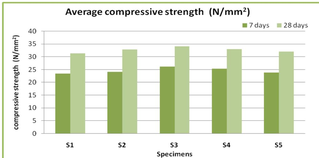
**Figure 2 Average compressive strength of GPC**
