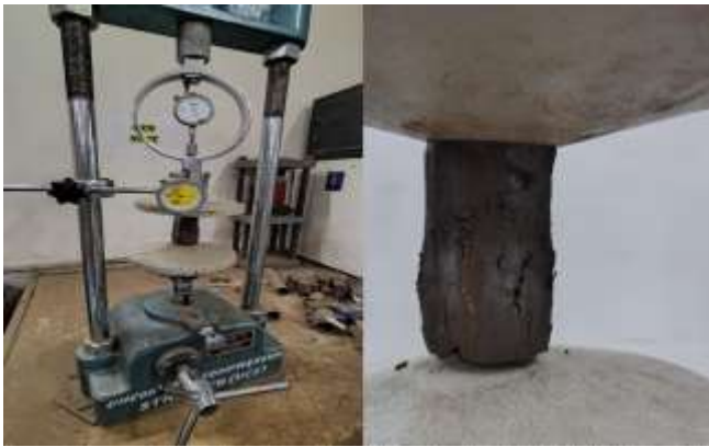
Figure 1.5 UCS test Apparatus and sample testing
