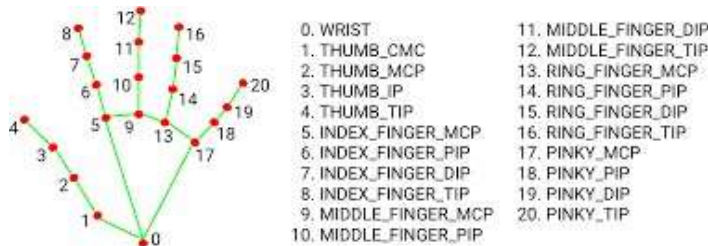
Fig -2: Hand Landmark Representation.
