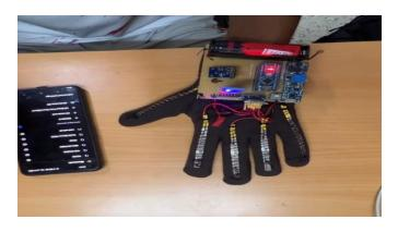
Making The Gestures & Observing The Output: Once both the devices are successfully connected, open the Arduino speech to text converter application on the android device. Look for the Bluetooth module HC-05 in the list and tap on it. Once it shows connected, start making the gestures for which the commands are saved. For every gesture that has been made, the phone will display the respective command and read it out loud too.
