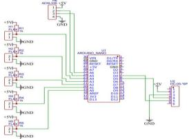
**Flex Sensor:** Flex sensors play the major role in Gesture Vocalizer. Flex sensors in gesture vocalizer is used as bend sensors. We connect the flex sensors at each finger of hand. Flex sensors are used to detect the bending of fingers. We are using the flat resistance of 10K. the voltage varying between 0-5 volt. As the bending of finger is minimum the voltage at output is maximum that is 5v and vice versa. The resistance value is converted into voltage.
