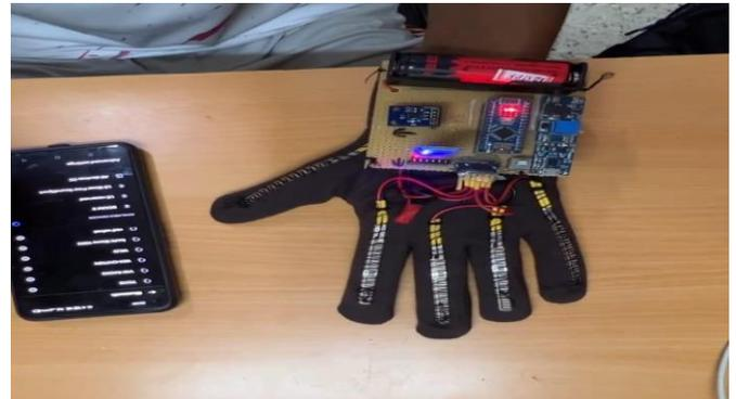
**Making The Gestures & Observing The Output:** Once both the devices are successfully connected, open the Arduino speech to text converter application on the android device. Look for the Bluetooth module HC-05 in the list and tap on it. Once it shows connected, start making the gestures for which the commands are saved. For every gesture that has been made, the phone will display the respective command and read it out loud too.
