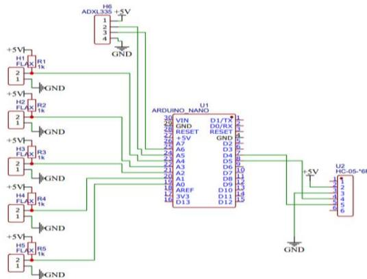
**Flex Sensor:** Flex sensors play the major role in Gesture Vocalizer. Flex sensors in gesture vocalizer is used as bend sensors. We connect the flex sensors at each finger of hand. Flex sensors are used to detect the bending of fingers. We are using the flat resistance of 10K. the voltage varying between 0-5 volt. As the bending of finger is minimum the voltage at output is maximum that is 5v and vice versa. The resistance value is converted into voltage.
