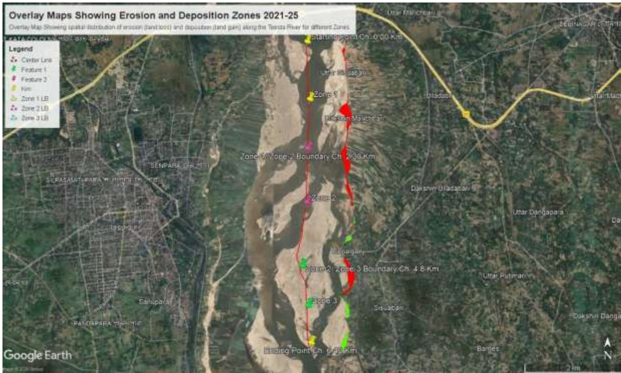
Figure 8: Spatial distribution of erosion (bank retreat) and deposition (sediment accumulation) zones along the Teesta River reach derived from overlay analysis of bankline positions between 2021 and 2025.
