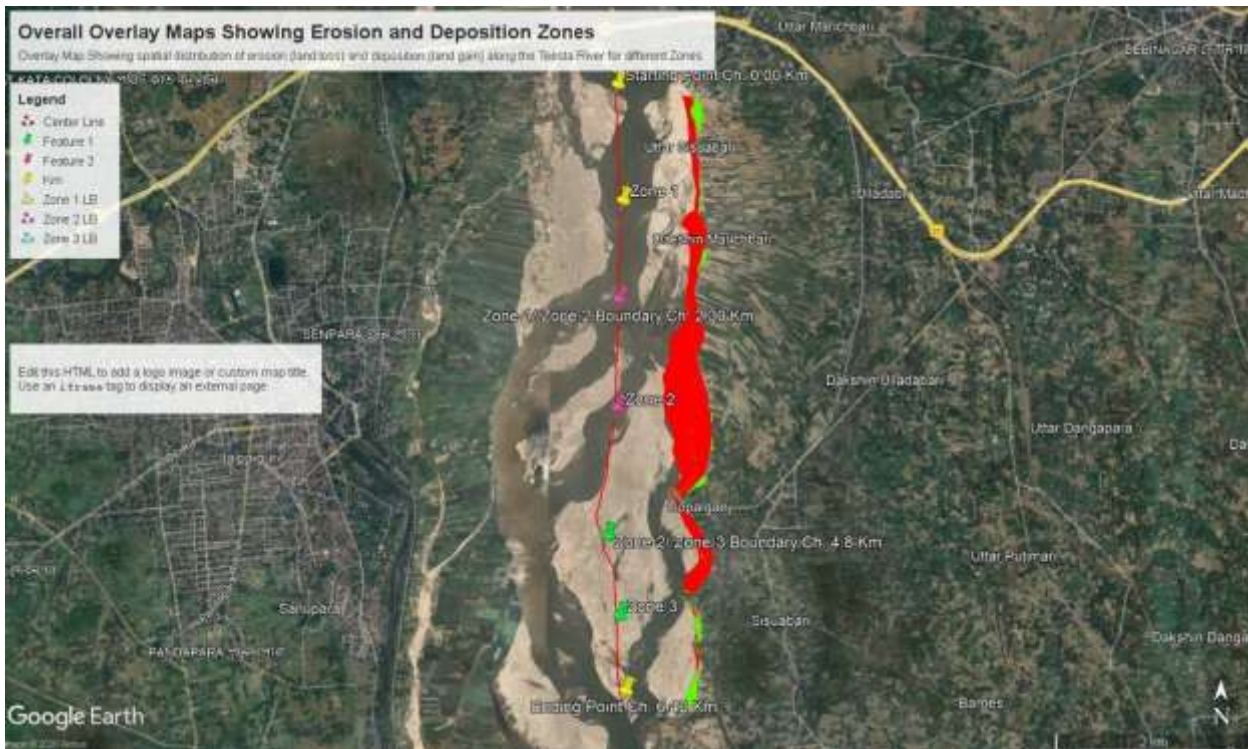
Figure 9: Overall spatial distribution of erosion (bank retreat) and deposition (sediment accumulation) zones along the Teesta River reach based on multi-temporal overlay analysis (2011–2025). The figure presents the overall spatial distribution of erosion and deposition zones along the selected reach of the Teesta River based on multi-temporal
