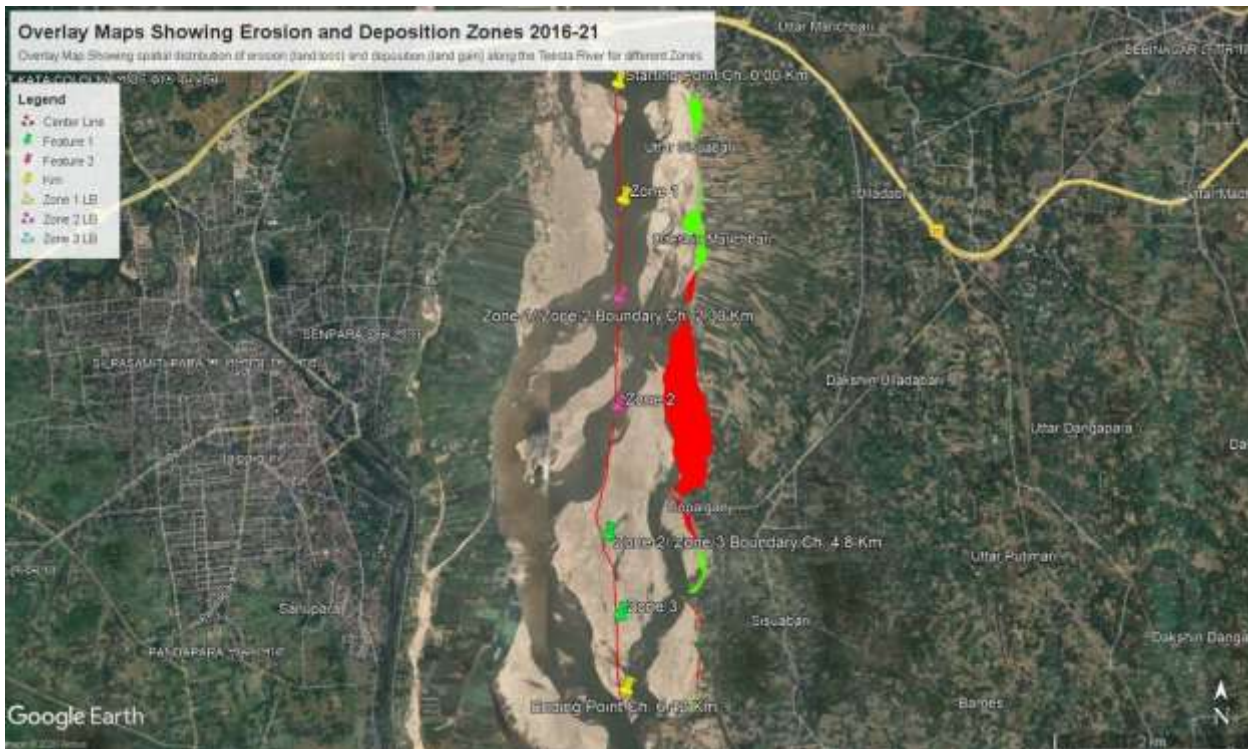
Figure 7: Spatial distribution of erosion (bank retreat) and deposition (sediment accumulation) zones along the Teesta River reach derived from overlay analysis of bankline positions between 2016 and 2021.
