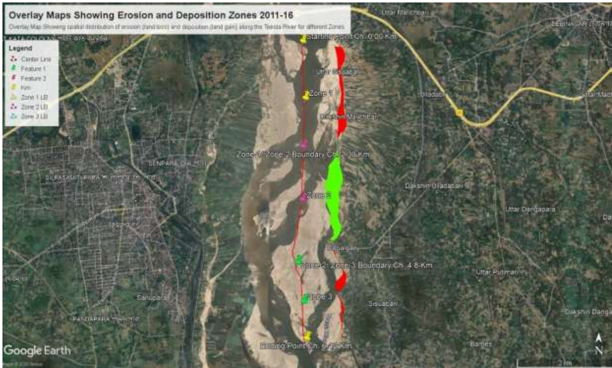
Figure 6: Spatial distribution of erosion (bank retreat) and deposition (bar formation) zones along the Teesta River reach derived from overlay analysis of bank line positions between 2011 and 2016.
