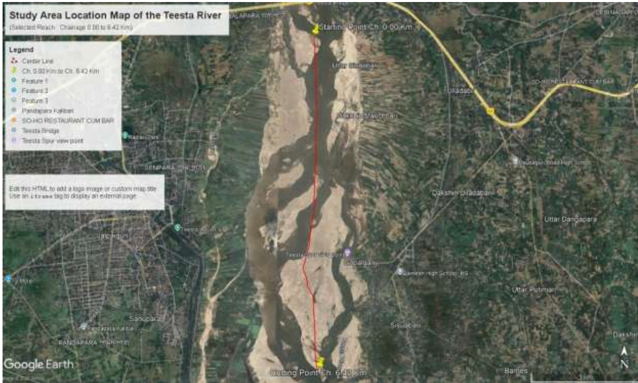
Figure 4: Study area location map of the selected Teesta River reach showing the centerline alignment, chainage from 0.00 km to 6.42 km, and key reference points including starting and ending locations used for morphodynamic analysis.
