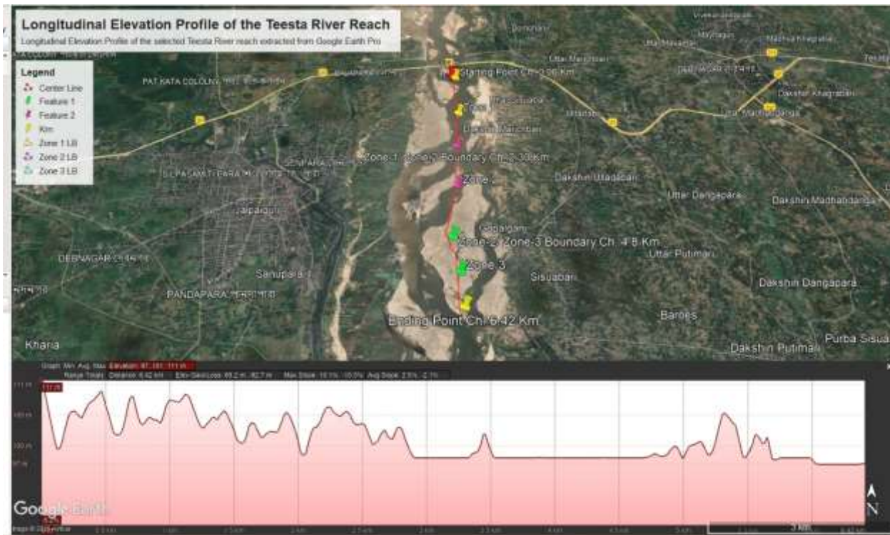
Figure 2: Longitudinal profile and planform of the selected Teesta River reach showing elevation variation, channel alignment, and zonation into three morphodynamic reaches (Zone 1, Zone 2, Zone 3) based on slope characteristics.
