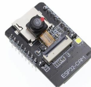
Fig.6.ESP32 Cam Module for the license Plate Recognition.
