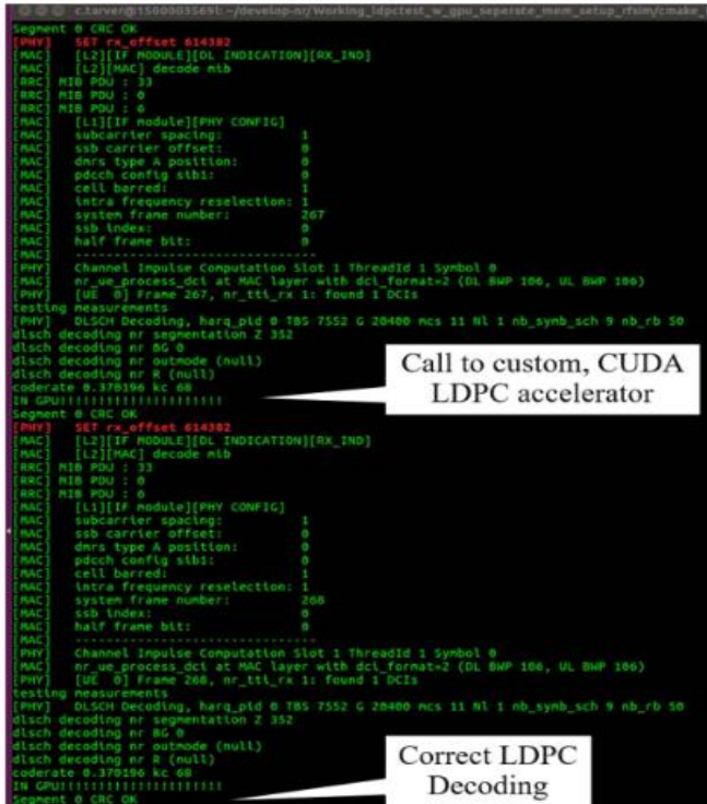
FIGURE 10. Example calling the custom, LDPC accelerator from the OAI ldpctest.
