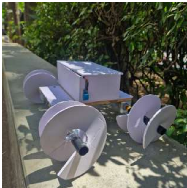
Fig. 5. Assembled Grain Silo Robot — External View
