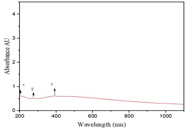
The uv visible light at wavelength ranging from 200-800 nm was used to evaluate the light absorption characteristics of TiO<sub>2</sub> nanoparticles. The UV visible spectra of TiO<sub>2</sub> and leaf extract in an aqueous solution at room temperature. The absorption peaks obtained for the samples in the range of 203.25 nm for titanium dioxide. For the peak 289.75nm the corresponding absorption range is 0.6139AU.
