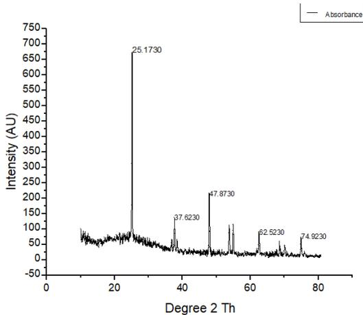
Using X ray diffraction phase analysis was studied. The average crystalline size of the nanoparticles were calculated based on Debye' scherer's equation.
