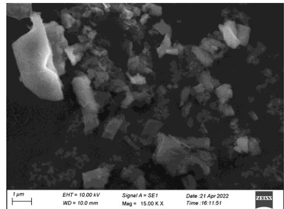
SEM image of TiO<sub>2</sub> for 1 $\mu$ m
