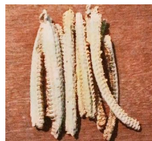
Fig. 3. Filter Media by using corncobs
