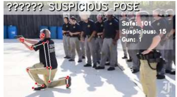
Figure 6 Example outputs from the real-time threat detection system
