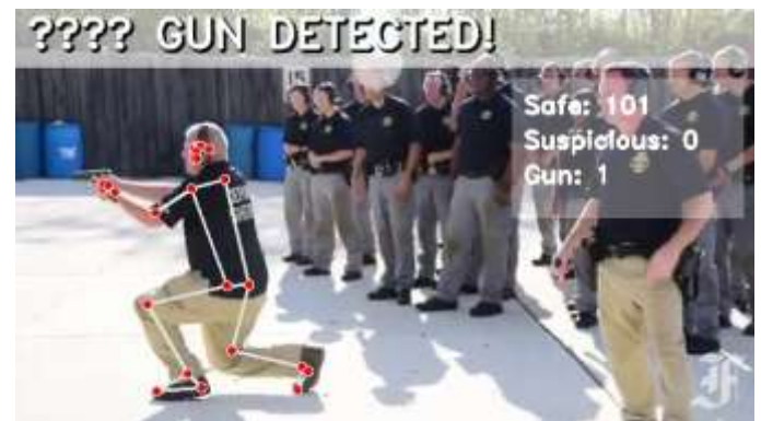
Figure 7 Example outputs from the real-time threat detection system
