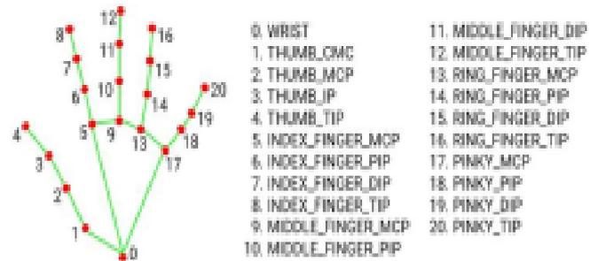
Fig 2. MediaPipe Structure
