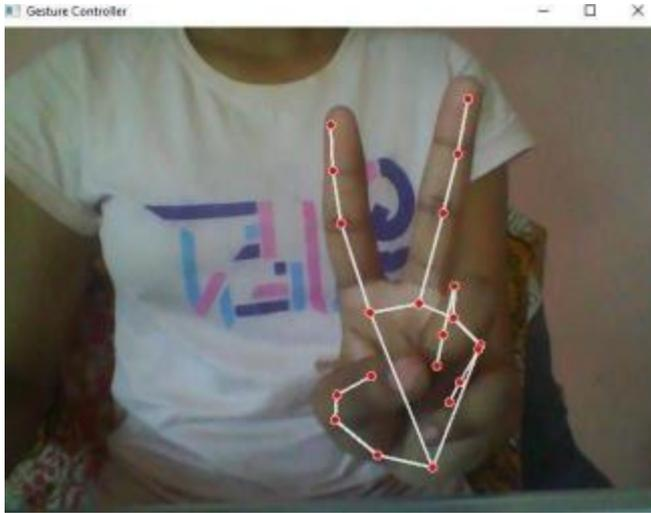
**Fig.3 Gesture for Moving the Mouse**
