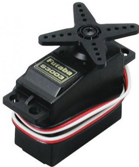
Fig. 9 – Servo Motor used for Seed Dispensing
