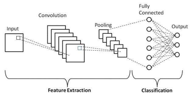
Figure 2. Typical convolutional neural network architecture.
