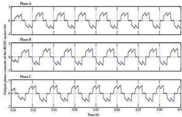
**Figure 10.3** Output waveform of BLDC motor
