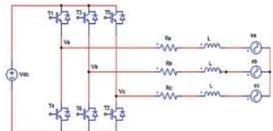
Figure 8.1 Equivalent circuit diagram of BLDC motor
