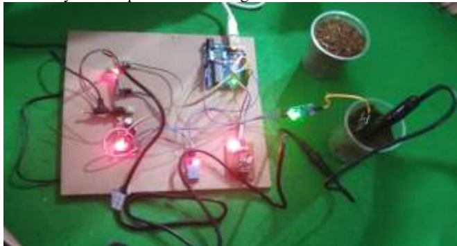
Fig 1. Collect values by inserting NPK sensor into soil.
