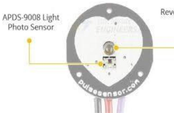
Just below the LED could be a small ambient light photo sensor – [APDS-9008 from Avago](#), almost like that employed in cell phones, tablets and laptops, to regulate the screen brightness in different light conditions
