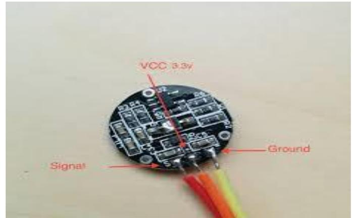
b) Pulse Sensor: The front of the sensor is that the side with the center logo. This is often where you place your finger. On the front side you may see a little round hole, from where the Kingbright’s reverse mounted green LED shines.
