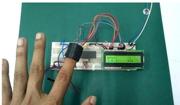
the module of the Microcontroller circuit which may be a media interface for data digital communication between the Arduino Uno and smartphone in an exceedingly real time. The brief description as follows:
