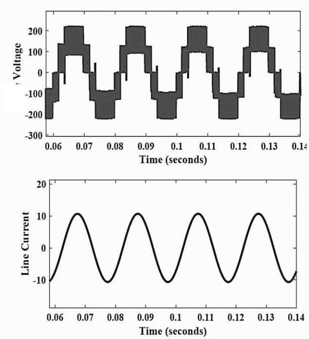
Fig. 5. Three level Capacitor clamped voltage and current waveforms.
