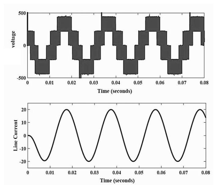
Fig. 7. Voltage and current waveforms of three level cascaded inverter.
