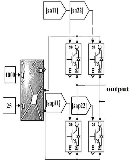
Fig. 6. Three level Cascaded PV source model in MATLAB/simulink.
