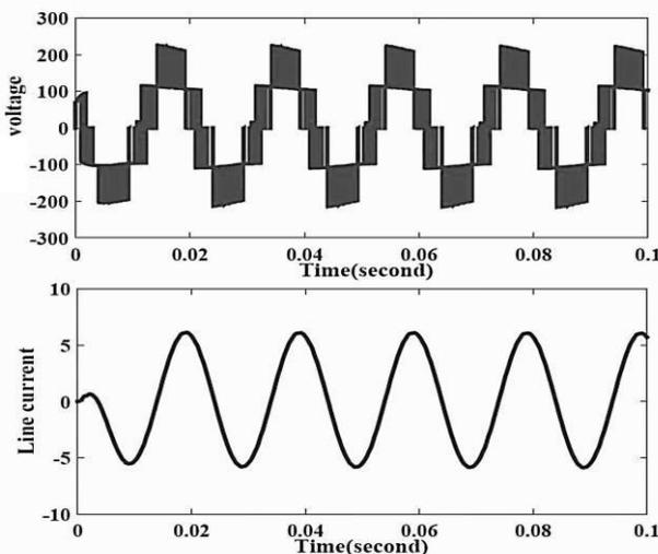
Fig. 13. Voltage and current waveforms of three level hybrid model.
