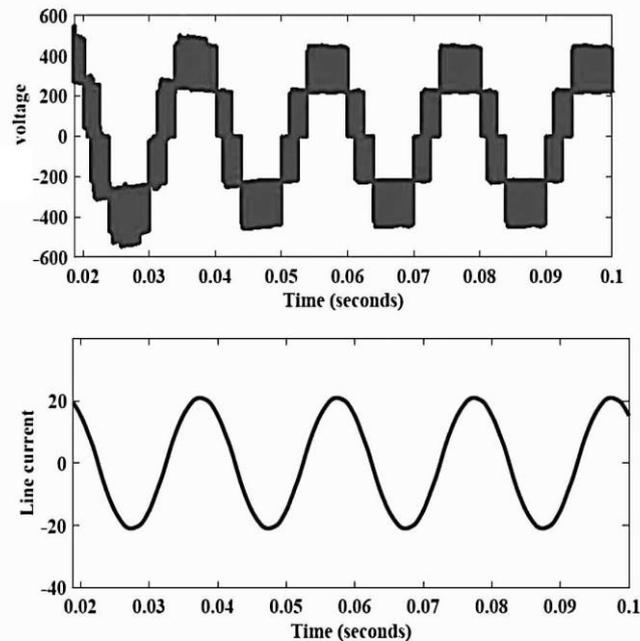
Fig. 11. Voltage and current waveforms of three level Quasi Z source.
