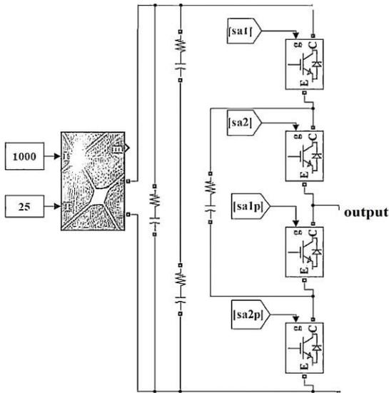
Fig. 4. Three level Capacitor clamped, PV source model in MATLAB/Simulink.
