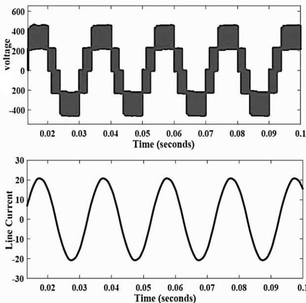
Fig. 9. Voltage and current waveforms of three level Z source inverter.
