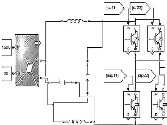
Fig. 8. Three level Z-source PV connected inverter in MATLAB/simulink.
