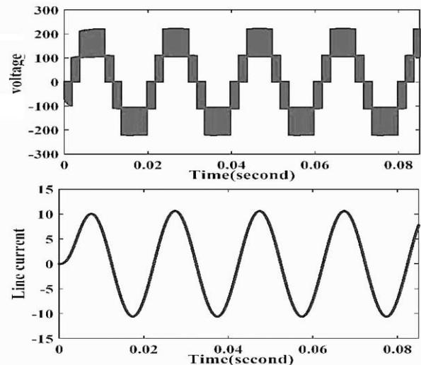
Fig.3. Three level NPC inverter voltage and current waveforms.
