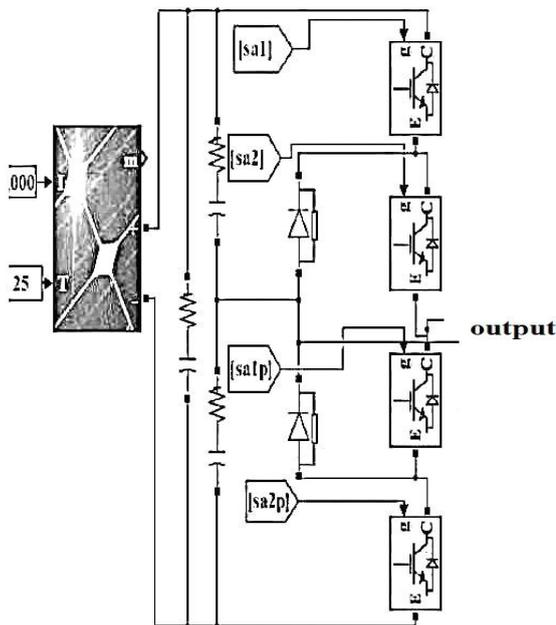
Fig. 12. Three level Hybrid PV source inverter in MATLAB/simulink.
