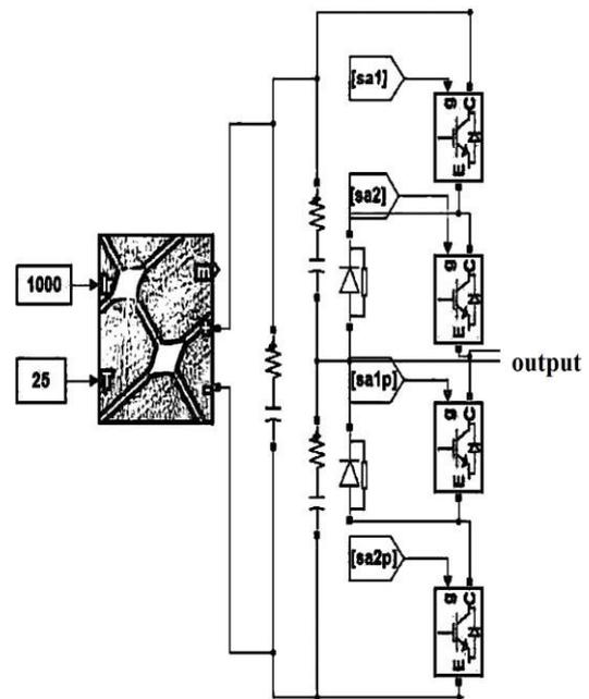
Fig.2: Threelevel NPC, PV source model in MATLAB/Simulink.
