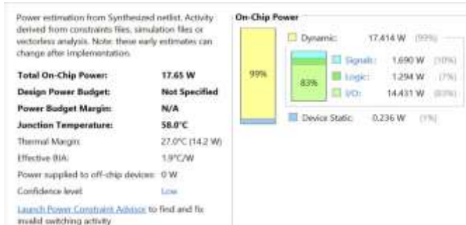
Fig.2: Power Report of 8-bit MAC with Ripple Carry Adder
