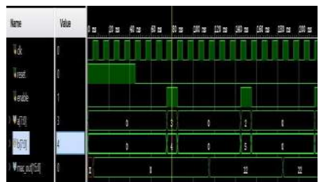
Fig.13 : Simulation results of 8-bit MAC with Brent Kung Adder
