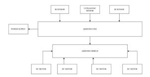
Firstly, the hardware components need to be assembled. This includes connecting the IR and ultrasonic sensors to the Arduino shield, ensuring proper wiring and compatibility. The Arduino shield acts as the central control unit, allowing for seamless integration and communication between the sensors and the microcontroller.
