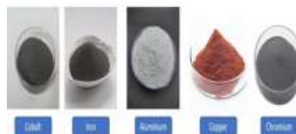
Fig. 2 — Reinforcement Powders: Co, Fe, Al, Cu, Cr (1.8 wt.% each)
