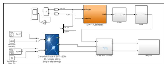
**Fig 1: Proposed framework for MPPT Controller**
