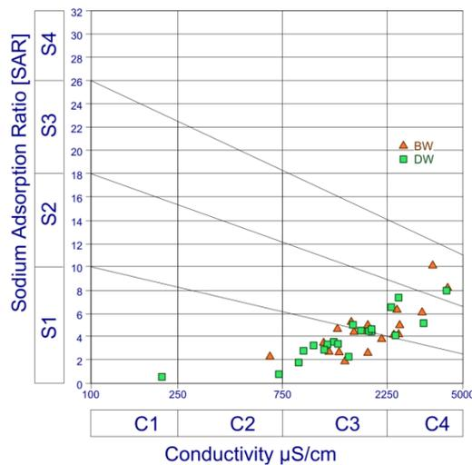
Fig. 4 Salinity and Sodium Adsorption Ratio (after USSL 1954)
