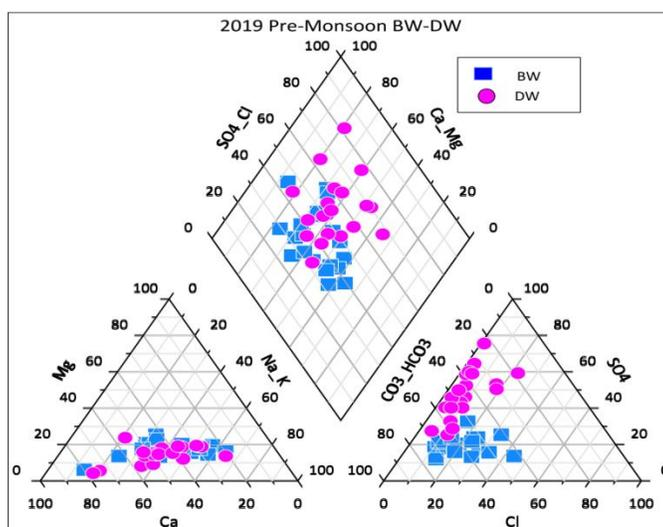
Fig 3: Piper Classification for water types
