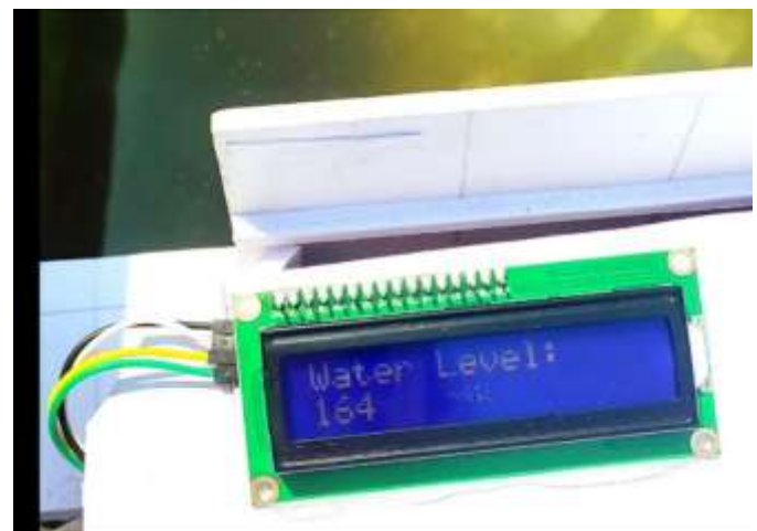
Fig 11: Depth Indication when placed in Water
