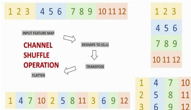
**Fig-3:** Channel Shuffle Operation
