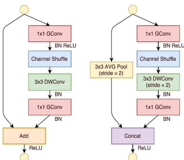
**Fig-5:** (a) the basic unit of ShuffleNet v1, (b) the basic unit for scaling down in ShuffleNet v1
