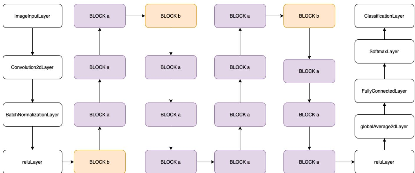
**Fig-4:** ShuffleNet Block Diagram
