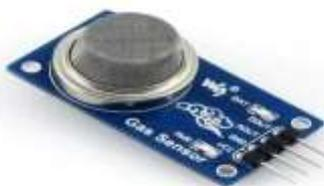
**Fig 7:** MQ 2 In 1 Sensor
