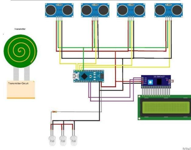
Fig.3 Circuit diagram (Transmitter)
