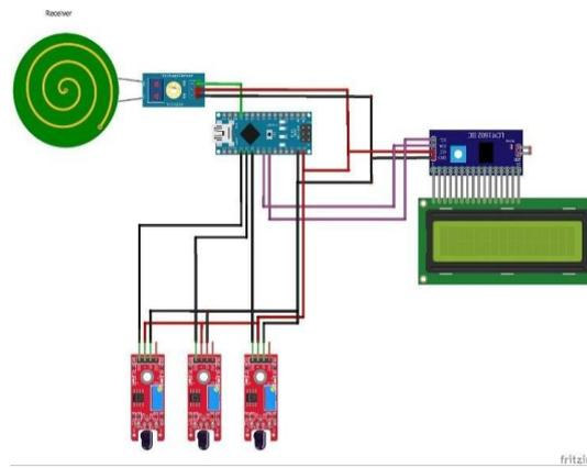
Fig.4 Circuit diagram (Receiver)
