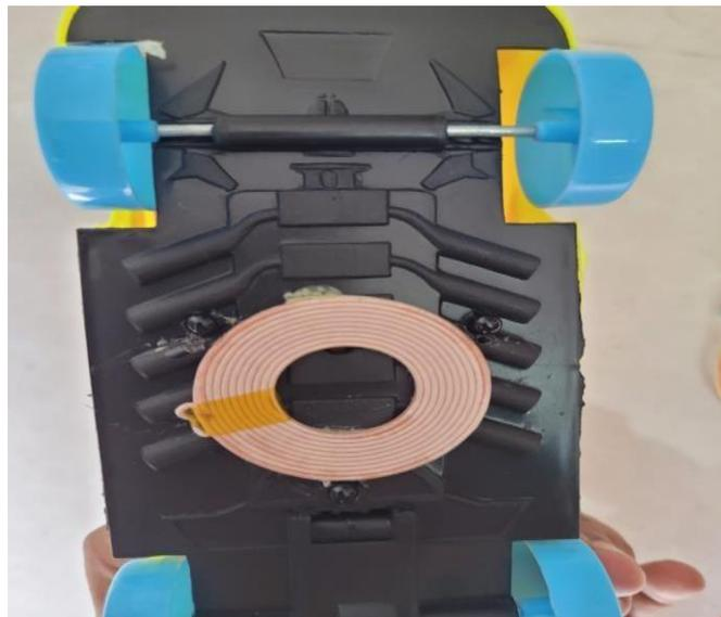
Fig:6 Secondary receiver coil on vehicle
