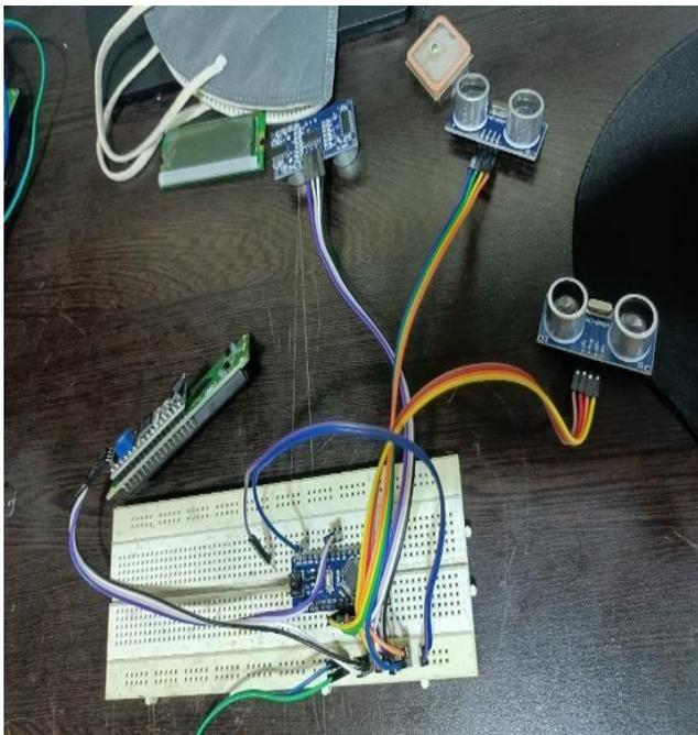
Fig.8: Testing of ultra-sonic sensors
