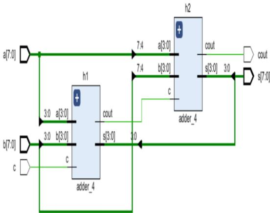
Fig.1 8 Bit Schematic Diagram
