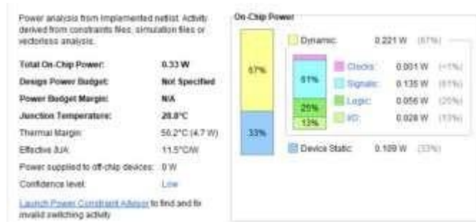
Fig-8: Power analysis of five stage pipelined RV32I RISC-V core
