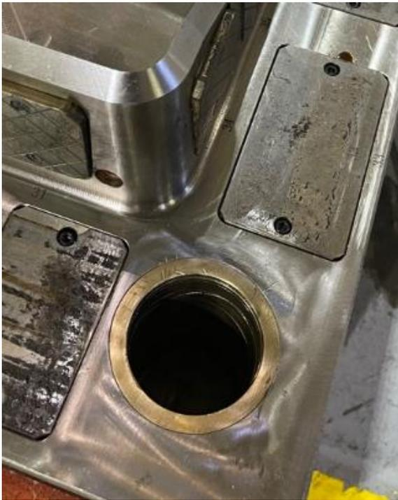
(Figure 4: Shows the Brass-Bushing we installed.)
