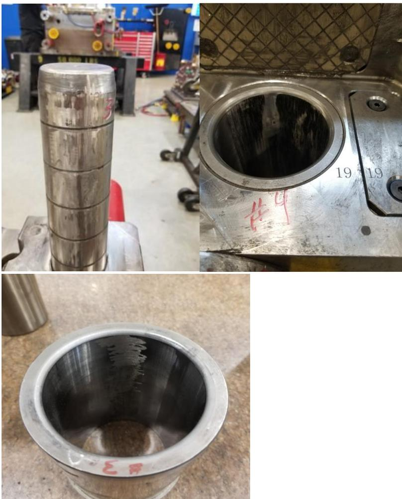
(Figure 1, 2 and 3: Steel Pin and Steel-Bushings showing Excessive wear due to Friction)
