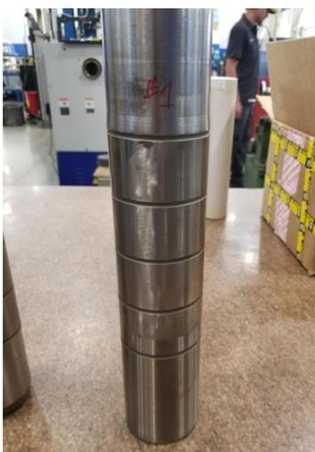
Figure 5: Polished the Steel-Pin before re-installing back into the Mold.
