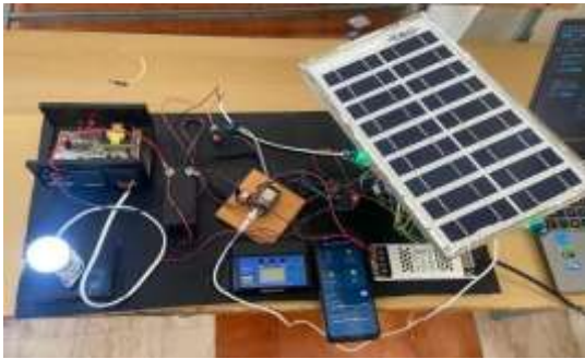
Figure 4.2 : Real-Time Hardware Implementation of Dual Axis Solar Tracking
