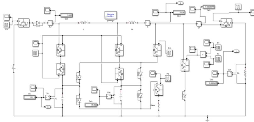
Here, Multi-sectioned model is presented, where number of sections is varied in order to compare the difference in output waveforms. An input of 6kV was given, for a load of 10 ohms. All the sub-systems are single staged but with varying number of sections. The Output in shows that as we increase the no. of sections, the pulse-width increases. But there is no difference in output voltage of the generator. As observed, increasing the number of stages, multiplies the output voltage.
