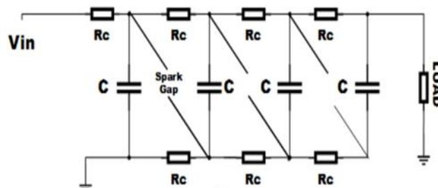
Fig.1 Schematic of four stage Marx generator
