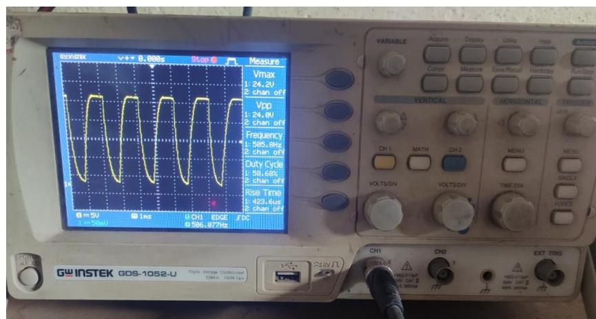
Fig.6.2: Waveforms of boosted voltage pulses of Marx generator
