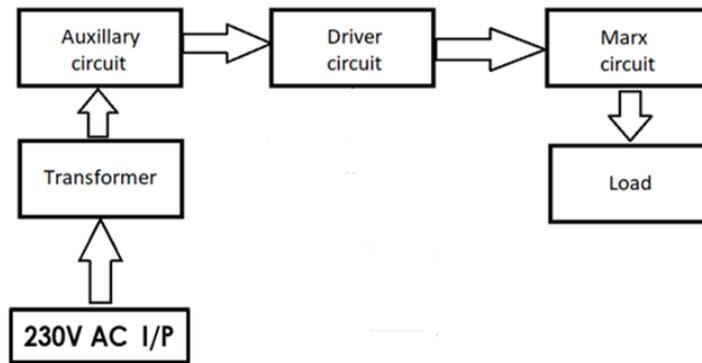
**Fig.5.3: Block diagram for Proposed Topology in Hardware**
