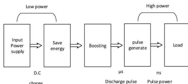
Fig.2.1: Block diagram of BCPFN Marx generator
