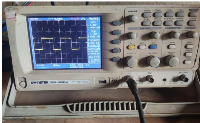
Fig.6.1: Waveforms for Triggering pulses of Marx generator
