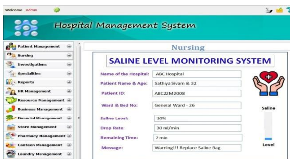
Fig-12: Patient Monitoring Database showing Warning Message and Alarm the Nurse to Replace the Saline Bag when 90% Saline Solution gets over
