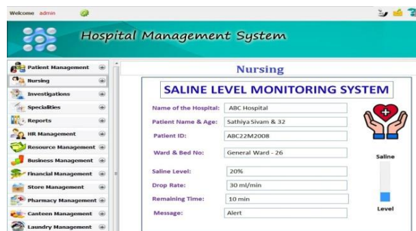
Fig-10: Patient Monitoring Database showing Alert Message when 80% Saline Solution gets over
