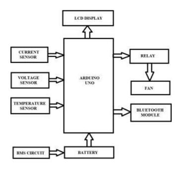
An electric vehicle's real-time battery monitoring system is implemented using a simple block diagram approach.
