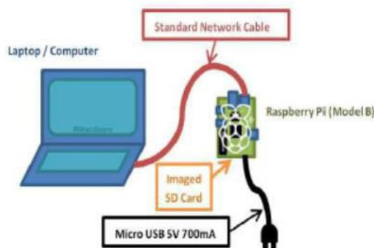
Figure 3. Raspberry Pi Connections
