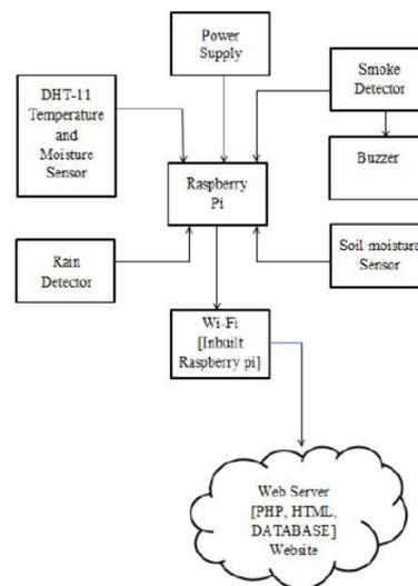
Figure 1. Block diagram of Green House Monitoring System
