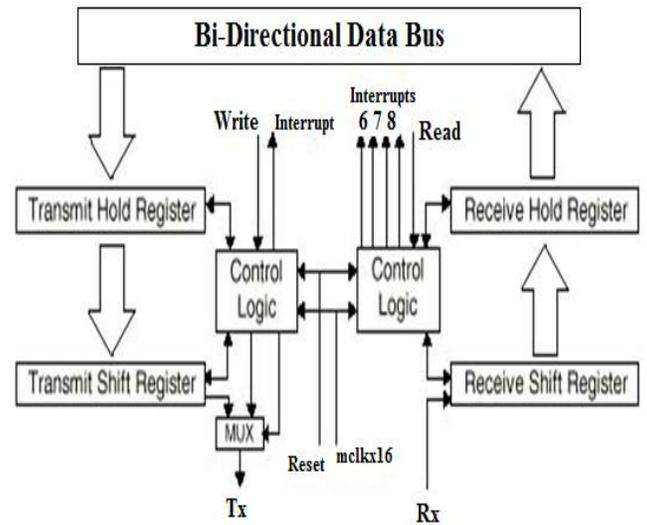
Figure: Block diagram of bi-directional UART
