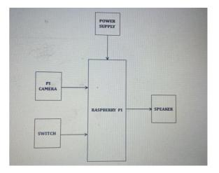
The basic working of the prototype can be given as capturing the images using OCR based raspberry pi module, conversion of the images into text by image processing, conversion of the text to speech using the Google text to speech (GTTS) converter and haptic feedback for orienting in-textline. The block diagram as shown. the Represents methodology. The acquisition of images from a book and recognizing printed text from the image is performed using Raspberry Pi
