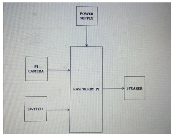
The basic working of the prototype can be given as capturing the images using OCR based raspberry pi module, conversion of the images into text by image processing, conversion of the text to speech using the Google text to speech (GTTS) converter and haptic feedback for orienting in-text-line. The block diagram as shown. Represents the methodology. The acquisition of images from a book and recognizing printed text from the image is performed using Raspberry Pi
