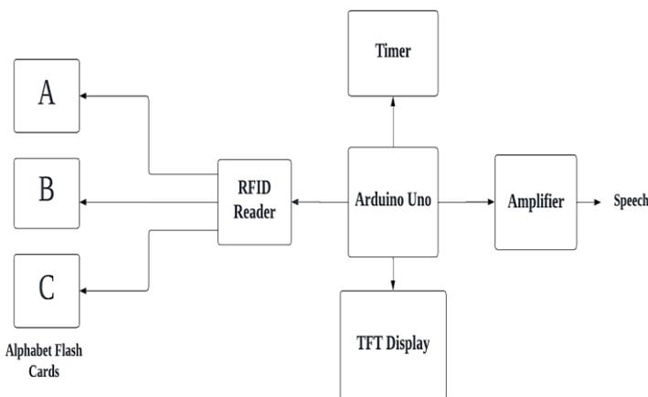
Fig.3 Proposed system block diagram
