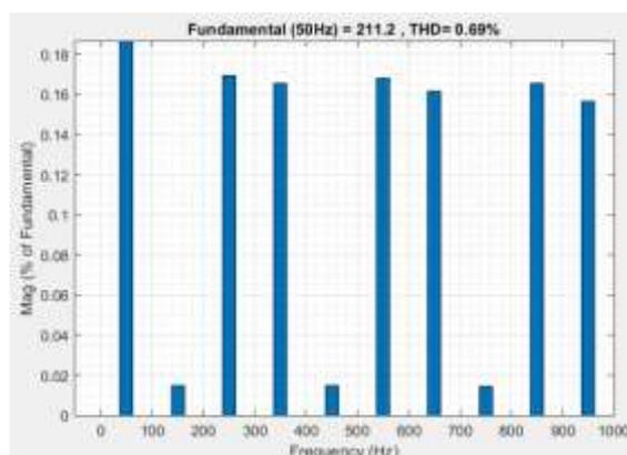
Figure 2. Graph of the source voltage
