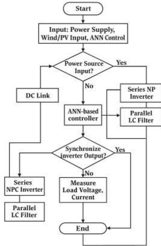
**Fig. 2: Process Flow chart of the Proposed Architecture**
