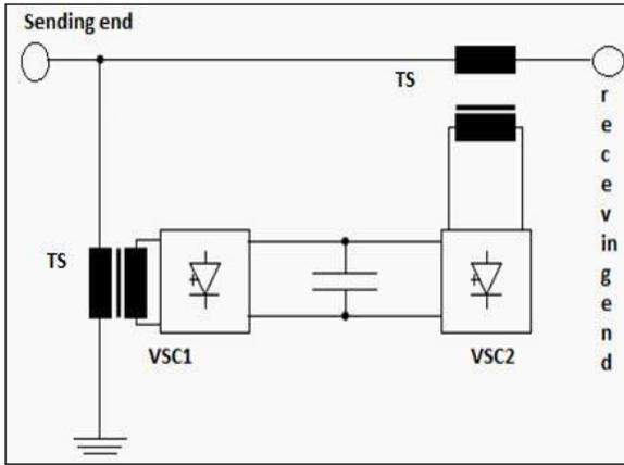
Figure 1: Basic diagram for UPFC
