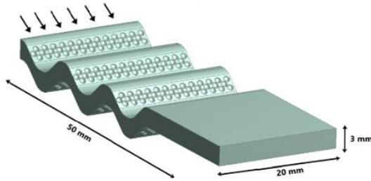
Figure 7 Geometric domain for the singular heat exchanger channel study.
