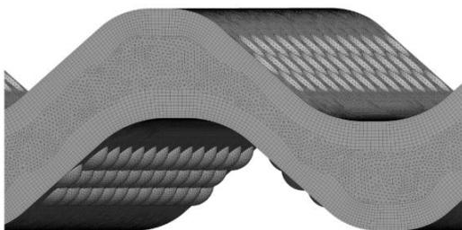
Figure 8 Dimpled single heat exchanger channel.
