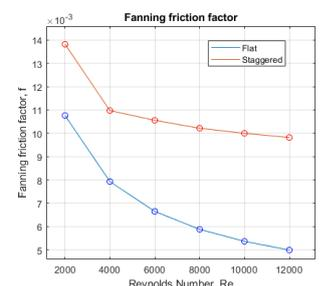
Graph 3 Heat transfer(left) and fanning friction factor(right) with dimples in a staggered arrangement (red line) and without dimples (blue line).
