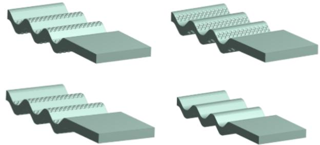
Figure 9 Four channel geometries with dimples placed at different positions.
