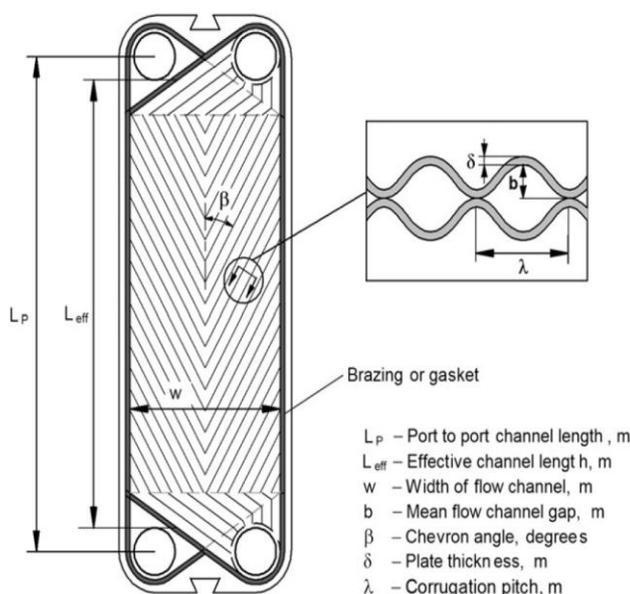
Figure 1.2 Herringbone pattern with corrugation angle  $\beta$  and illustration of flow channel geometry.
