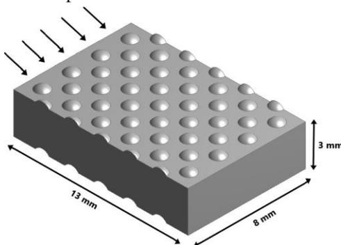
wide and 3 mm high and the fluid is flowing inside the rectangular domain from one short end to the other. The geometric domain as well as dimensions is presented in Figure 4.
