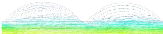
a close of a protruding dimple, which reveals a temperature maximum between adjacent protruding dimples. Bear in mind that a low temperature represents a region of high heat transfer, as this is where energy has been transported from the wall into the fluid. The regions of high and low heat transfer can be explained by studying the velocity field. The velocity field is presented in Graph 2.
